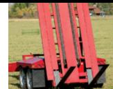
Strong and sturdy forks hold the bales in place while stacking and unloading.
