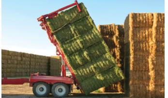
Once the bed is vertical, the alignment arms are opened, and the Bale Runner is driven forward to remove the forks from under the stack.
