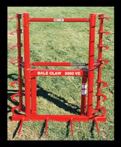
ProAG Bale Claw 5000VE The Bale Claw mounted to a loader moves bales easily from an existing stack to a truck, shed or bagger. The 5000VE will pick up three 3x3 bales, three 3x4 bales, or two 4x4 bales from the end of the stack for loading onto a truck.
