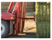
The 16K PLUS features a pushoff that when activated assists in moving the bales off the forks as you drive away.
