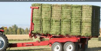
Computer controlled to maximize speed and to simplify your bale handling operation - to pick up and load bales, the operator toggles only the loader button. The computer determines the motion of the alignment arms, loader, grab hooks and power slider.
