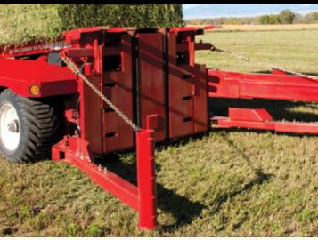
Bales are easily picked in any orientation. The alignment arms center the first bale - grab hooks hold the bale in place - the loader lifts slightly off the ground so the bale DOESN'T DRAG while traveling to the second bale. Stair stepping the bales during
