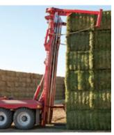
Steering with the hitch allows the operator to easily see and line up to the existing stack.
