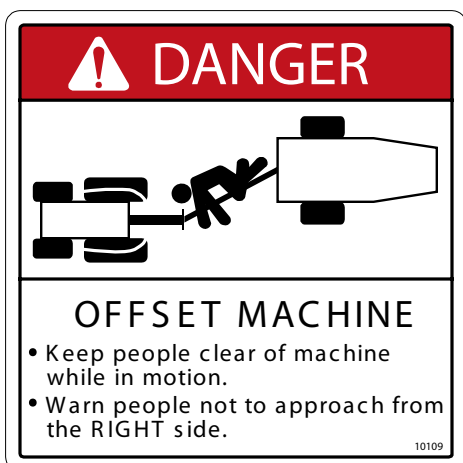
Part # 10109 - Danger Offset Machine Location: Right side of bed.
