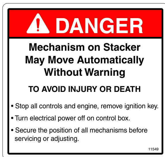
Part # 11549 - Danger Mechanism May Move Location: Top of hitch.
