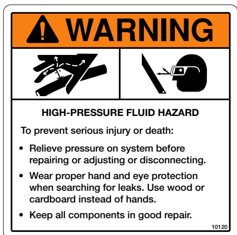
Part # 10120 - Warning High Pressure Fluid Location: Top of hitch.
