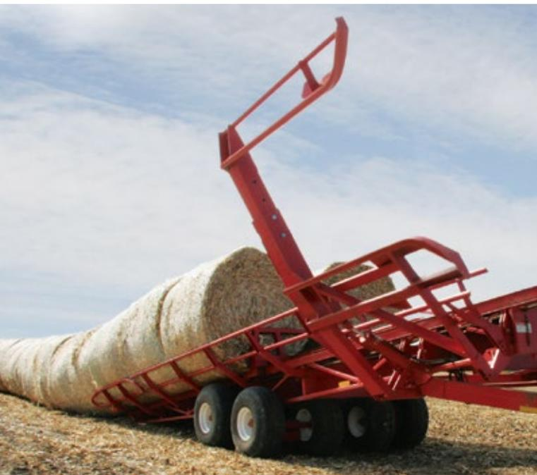
When unloading, the push bar travels all the way to the back, maintaining tight stacks. The adjustable bale divider has twelve positions to provide the operator the flexibility to set the bale spacing when unloading in the yard, providing the air circulation needed between the rows.
