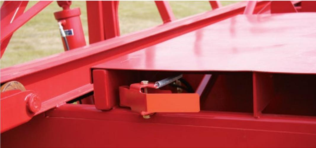
The full load indicator on the 2200 Bale Hiker signals the operator when the Bale Hiker has reached its maximum load capacity.
