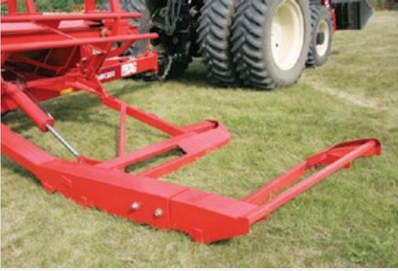
The robust heavy-duty bale fork adjusts to lift bales between 4 and 6 feet in diameter. Bale turners on the inside and outside of the fork allow bales to be picked in any direction. Right side picking reduces stress on the operator and eliminates weaving through the field.
