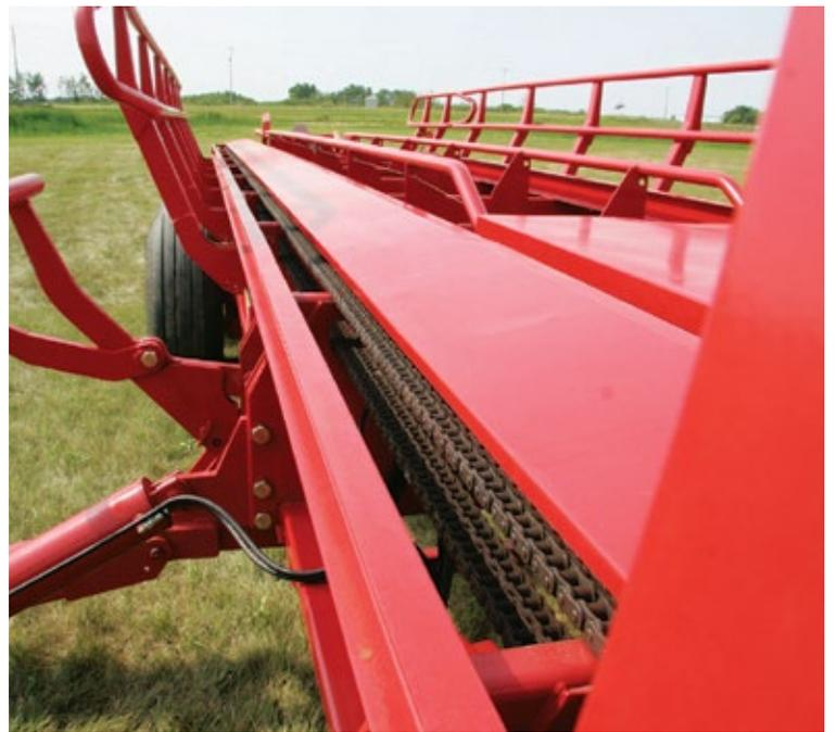
The smooth bed design protects net-wrap from tears, making it gentler than any other round bale carrier. Chains are completely covered and protected from dirt and debris that falls from the bales.
