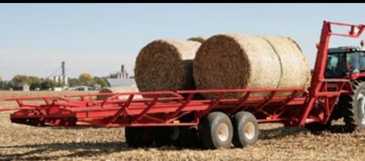
Only two hydraulic outlets are needed for full operation of the Bale Hiker.
