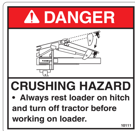
Part # 10111 Danger Crushing Hazard Location: Left side of Hitch.
