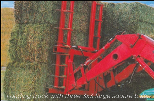
ProAG Bale Claw 5000VE The Bale Claw mounted to a loader moves bales easily from a stack to a truck. The 5000VE picks up three 3x3 bales, three 3x4 bales, or two 4x4 bales from the end of the stack for loading.
