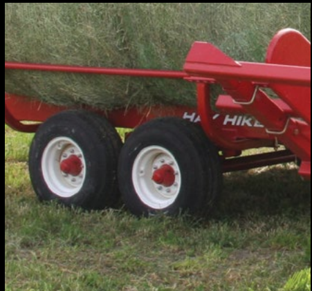
The 900 features heavy-duty axles, tires and 8-bolt hubs for exceptional load capacity.
