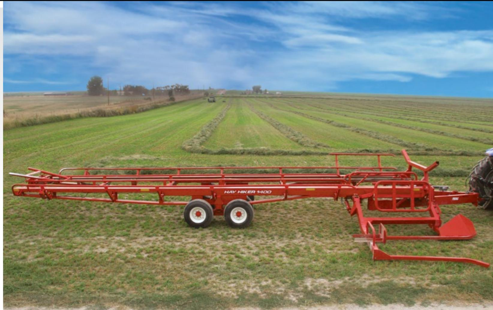
**Developed to fulfill the need for a simple, cost-effective round bale handling system...** The 900 and 1400 Hay Hikers are designed to quickly and efficiently move large round bales from field to storage (ProAG 1400 Hay Hiker shown).
