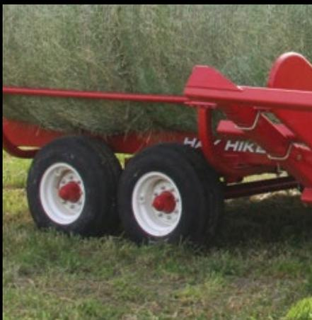
The 900 features heavy-duty axles, tires and 8-bolt hubs for exceptional load capacity.
