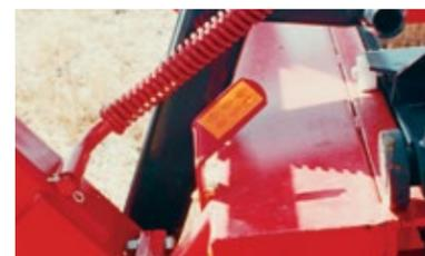
*The full load indicator on the 1400 signals the operator when the Hay Hiker has reached its maximum load capacity.*
