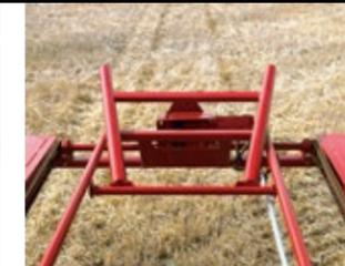
*The bale divider gently separates the bales as they are unloaded, creating air circulation between the two rows to prevent spoilage.*
