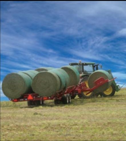
The 900 and 1400 are exceptionally well balanced to ensure safety and stability in transport. The heavy duty undercarriage enables the Hay Hiker to carry larger payloads and gives a smoother ride even in rough field conditions. The compact design lets you get to the next field quickly. The Hay Hiker's innovative pick on-the-go system, larger payload, compact transport design and single operator load/unload system provide a round bale handling system that saves time, fuel and labor.
