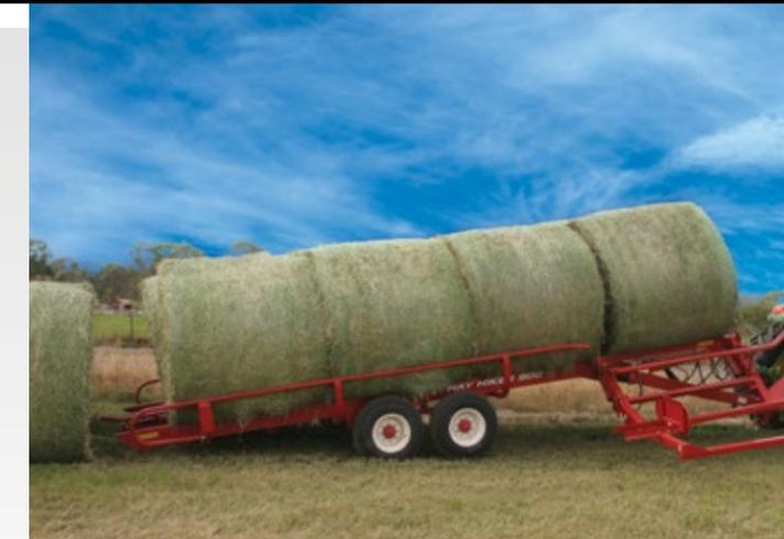
Handle bales from field to storage without leaving the tractor seat. The hydraulic control system tilts the frame bed to the ground while the push bar pushes the bales off the bed. As unloading progresses, the Hay Hiker moves forward slowly to allow the bales to settle on the ground.
