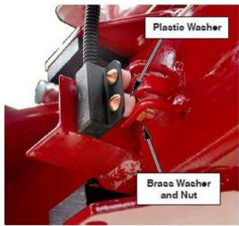
Ferrous Metal Sensor Mounting
