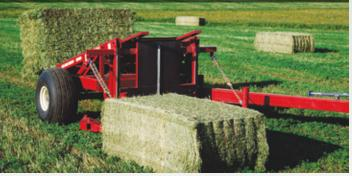
Bales are easily picked in any orientation they are automatically positioned with the two alignment arms as the HD4SR moves forward. When the bale is squeezed between the arms the loader automatically rotates up - both operate
