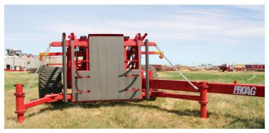
The Auto Align® system allows the operator to pick up bales in the same direction as the field was baled (12SR PLUS model shown).
