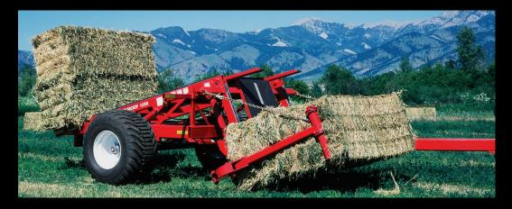
Automatic grab hooks hold the first bale in position, without dragging the bale, allowing the alignment arms to reopen to engage the second bale. The loader automatically rotates up as the two bales are squeezed. Bales can be picked in any orientation. The loader, alignment arms, and grab hooks are sequenced on one remote. Stair stepping the bales during loading aids in helping the bales slide back on the bed.
