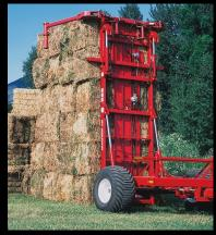
Once the bed is vertical, alignment arms are opened, and the 12SR PLUS is driven forward to remove the forks from under the stack.
